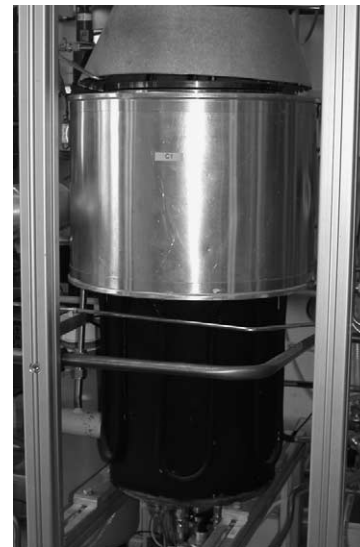
Fig. 1. The steam reformer. Approximate dimensions are 60 cm height and 28 cm diameter.
